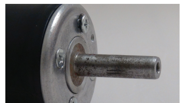
6. Putting screws back in place. Note diagonal tightening of screws.
