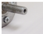
5. Hoof buffer with new bladder properly covering end of buffer.
