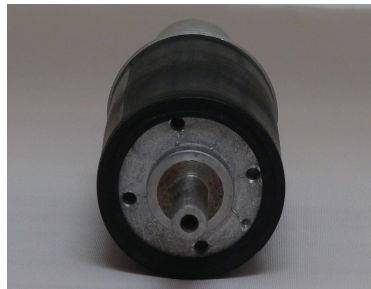
5. Hoof buffer with new bladder properly covering end of buffer.
