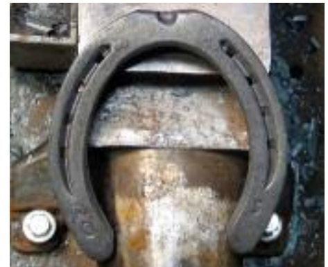
Finished clip from ground surface.
