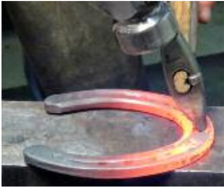
Bloom Wood Handled Bob Punch used to start source material for clip.
